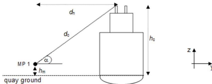
Figure 7. Sketch showing the relative position of the measurement position MP 1 to the funnel outlet of the auxiliary engine in operation.  $h_c$  is the height of the funnel outlet above quay ground,  $h_m$  is the microphone height above quay ground at the measurement position MP 1,  $d_h$  is the horizontal distance from MP 1 to the funnel outlet and  $d_c$  is the direct distance between the funnel outlet and MP1.
