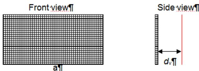
Figure 3. Sketch of a rectangular measurement surface for measuring the sound emission in front of a rectangular opening of a ventilation inlet or outlet. The contour of the measurement surface is marked red.
