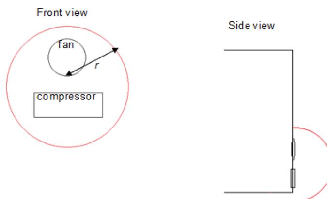
Figure 4. Sketch of the hemispherical measurement surface for measuring the sound emission of a cooled container. The contour of the measurement surface is marked red.
