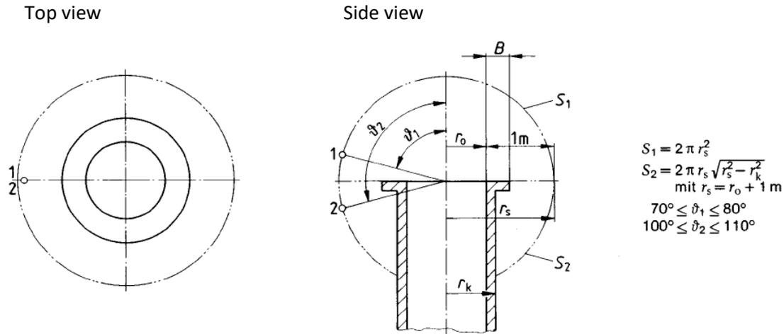
Figure 2. Measurement positions for measuring at the funnel outlet(s). The figure is taken from DIN 45635-47, Figure 1 [9].
