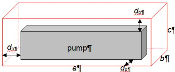
Figure 5. Sketch of the square measurement surface for measuring the sound emission of pumps. The contour of the measurement surface is marked red, the pump is marked grey.
